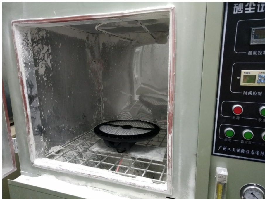
Photo 2: IP6X test of model A-CHB320
