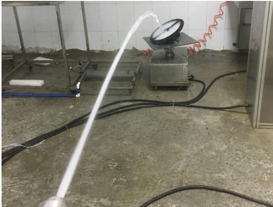
Photo 3: IPX5 test of model A-CHB320
